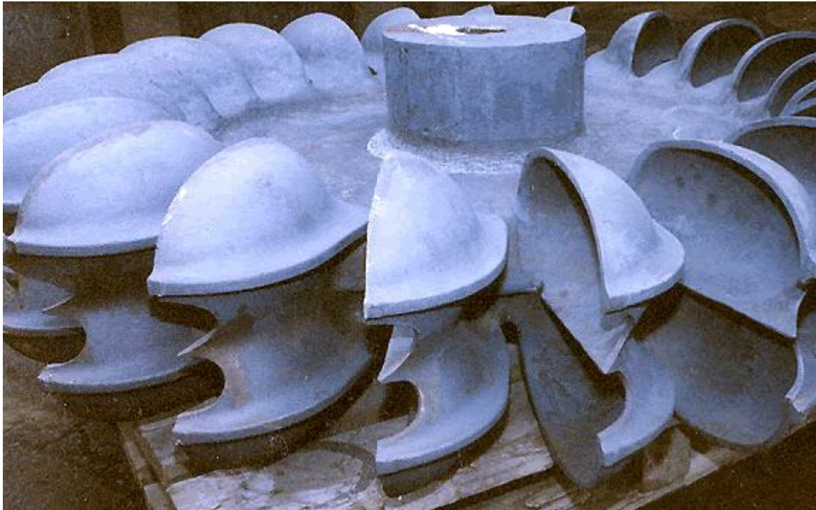
Figure Typical PELTON WHEEL with 21 Buckets
