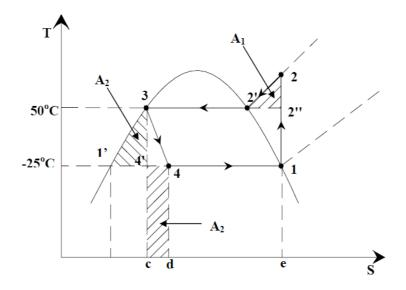
Using refrigerant R134a property data, required properties at various state points are:
