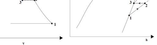
Fig.12.4(a) & (b): Intercooling in two-stage compression
