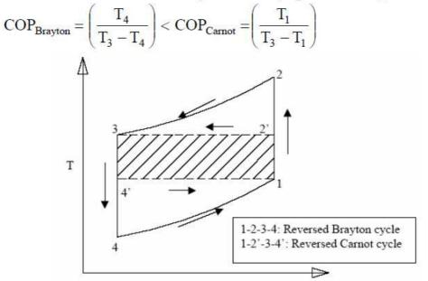
Fig. 9.3. Comparison of reverse Carnot and reverse Brayton cycle in T-s plane
