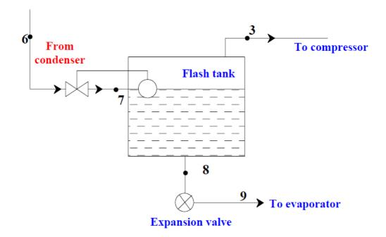
Fig.12.2(a): Working principle of a flash tank
