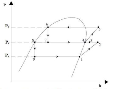
*Fig.126(b)*: Two-stage vapour compression refrigeration system with flash gas removal using a flash tank and intercooling – P-h diagram
