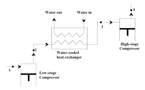
Fig.12.5(b): Intercooling using external water cooled heat exchanger
