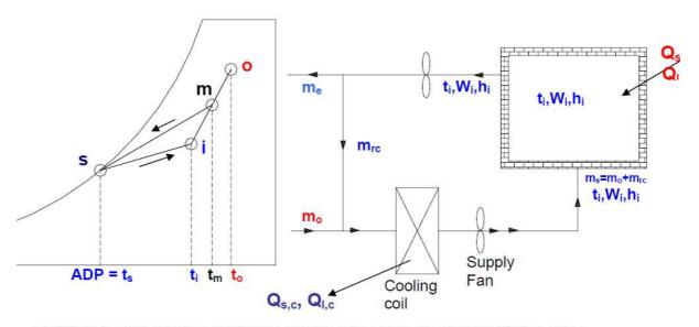
Fig.30.2: A summer air conditioning system with outdoor air for ventilation and a zero by-pass factor
