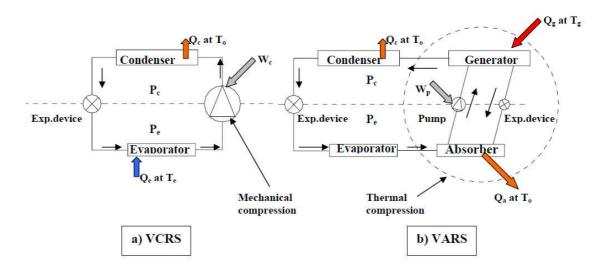
Figs.14.2: a) Vapour compression refrigeration system (VCRS) b) Vapour Absorption Refrigeration System (VARS)
