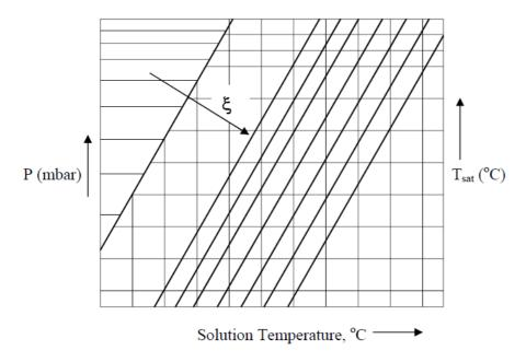
Fig.15.1.: A typical Dühring plot
