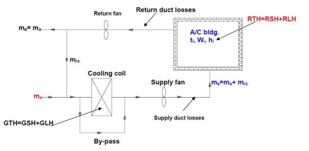
Fig.29.1: Schematic of a basic summer air conditioning system
