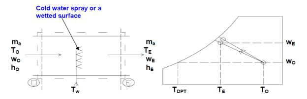
Fig.28.6: Cooling and humdification process
