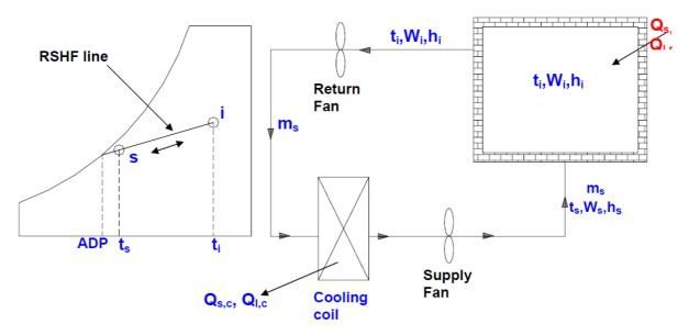
Fig.30.1: A simple, 100% re-circulation type air conditioning system
