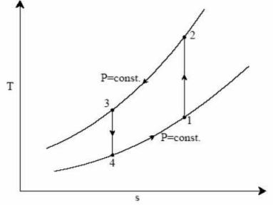
Fig. 2(b). Reverse Brayton cycle in T-s plane
