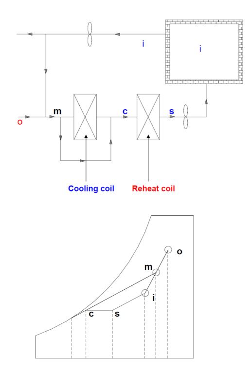
**Fig.30.4**: A summer air conditioning system with reheat coil for high latent cooling load applications
