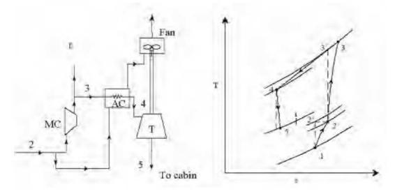
Fig. 9.5. Schematic of a simple aircraft refrigeration cycle
