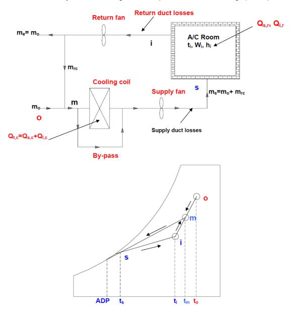
be seen from the figure that when X > 0, the room ADP will be different from the coil ADP. The system shown in Fig.30.3 is adequate when the RSHF is high ( > 0.75).
