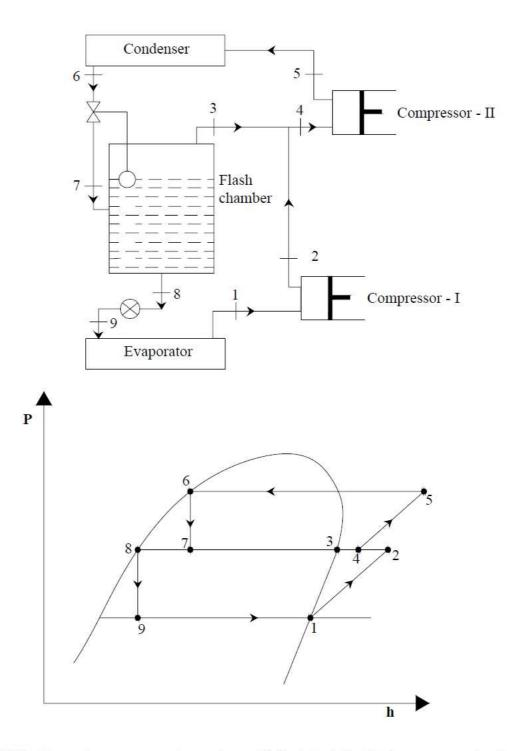
Fig.12.8: A two-stage compression system with flash tank for flash gas removal only (a) System schematic; (b) Cycle on P-h diagram
